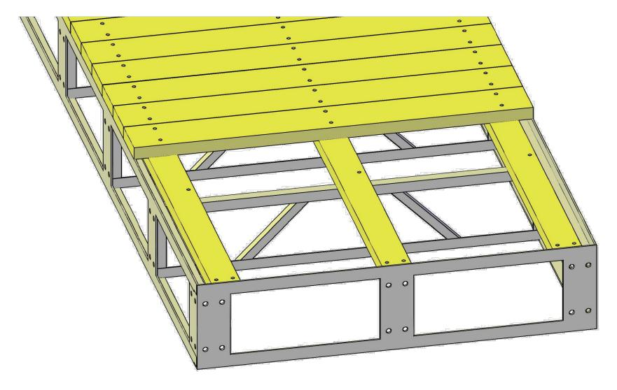
DECKING IS SECURED TO RUNNERS WITH 2-1/2" SCREWS FOR WOOD AND 2" SCREWS FOR COMPOSITE.
